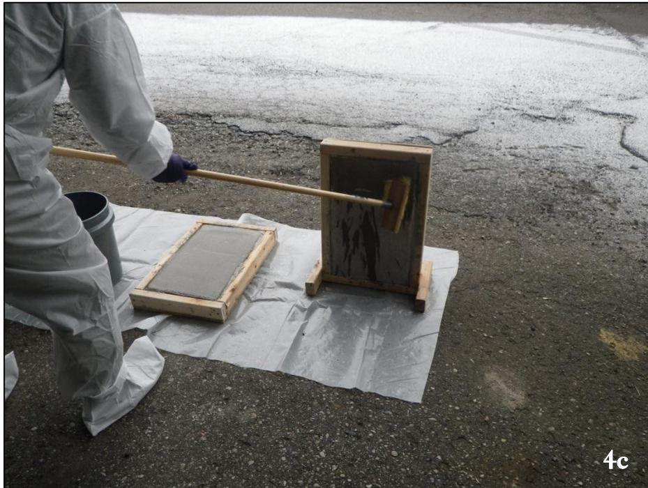
4. Simulated vertical wood stud surfaces, horizontal wood stud surfaces, horizontal wood sill plate surfaces, vertical OSB sheathing surfaces, horizontal concrete surfaces, and vertical concrete surfaces were contaminated with raw sewage. Sponge samples were collected from the contaminated surfaces.
