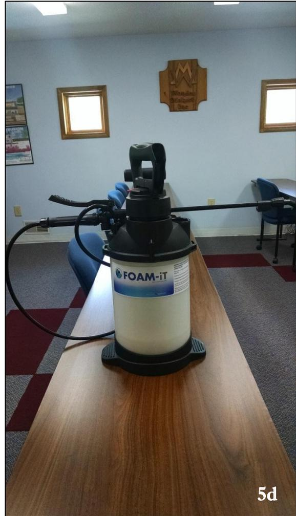
5. Following sponge sampling, the contaminated surfaces were sprayed with a diluted mixture of Atomic Degreaser using a FOAM-iT sprayer.
