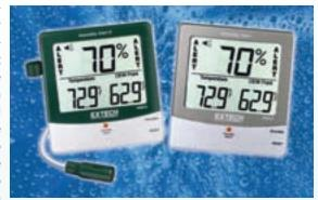
A large digit LCD screen allows for the simultaneous display of humidity, temperature and dew point. The meter measures humidity from 10 to 99 percent RH and temperature from 14° to 140° Fahrenheit.
